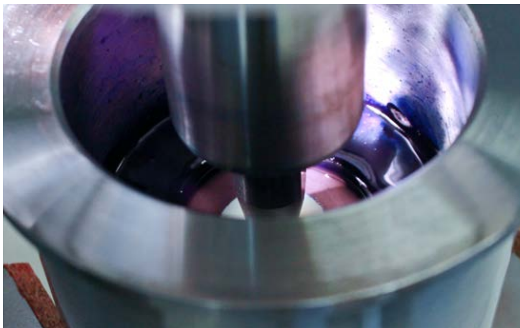
Perl mill for pigment grinding
